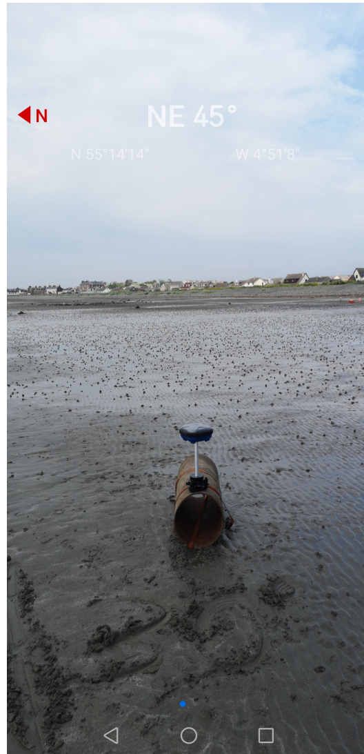
Figure 4.2: Target orientation. Instrument on top of the target is a high-precision GNSS North positioning unit.
