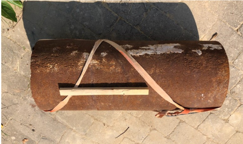
Figure 3.1: 50kg ferrous target used for the test. The rod on top is about 33cm long. Target dimensions: 75cm long with a diameter of 32cm.
